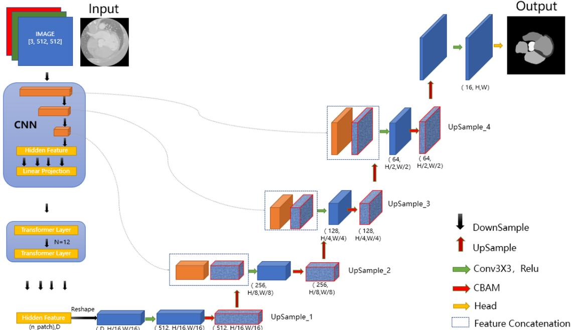
Fig. 3: The structure of TransNUNet [10]
