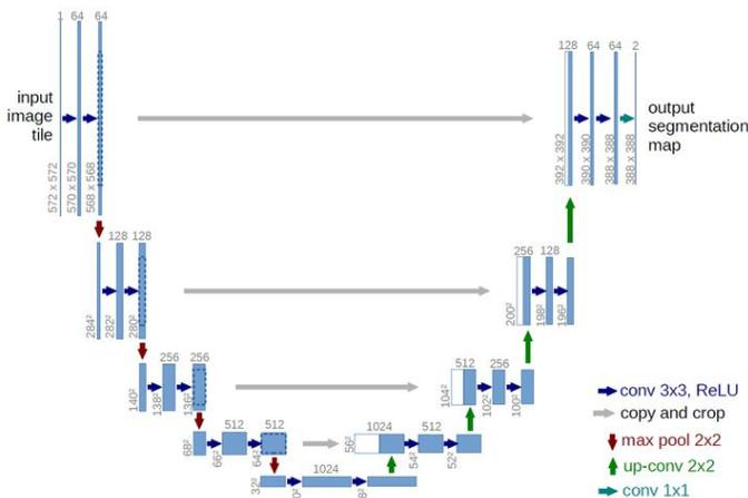
Fig. 1: The U-Net Architecture [1]
